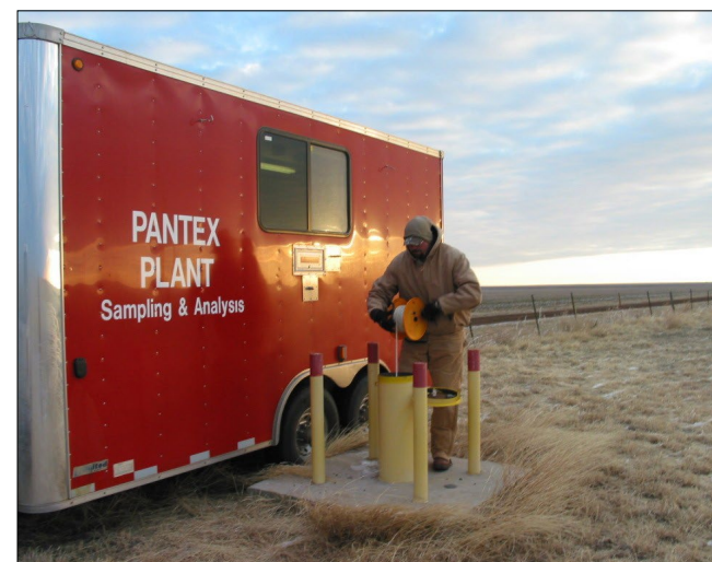
Sampling technician measuring depth to water
