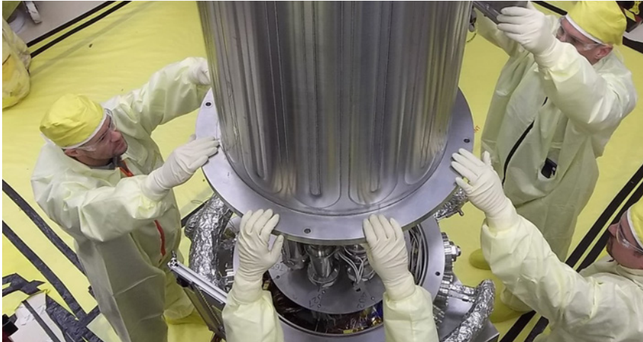
NASA is partnering with Y-12 and others on a reliable, efficient, kilowatt-size fission power system for future space missions. The prototype system is fueled with highly enriched uranium alloy components produced at Y-12. (Photo courtesy of NASA)
