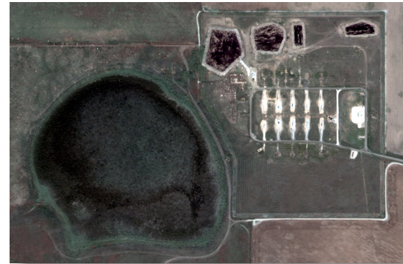
Newly installed landfill covers appear black in this June 2005 photo of the Burning Ground and Playa 3.
