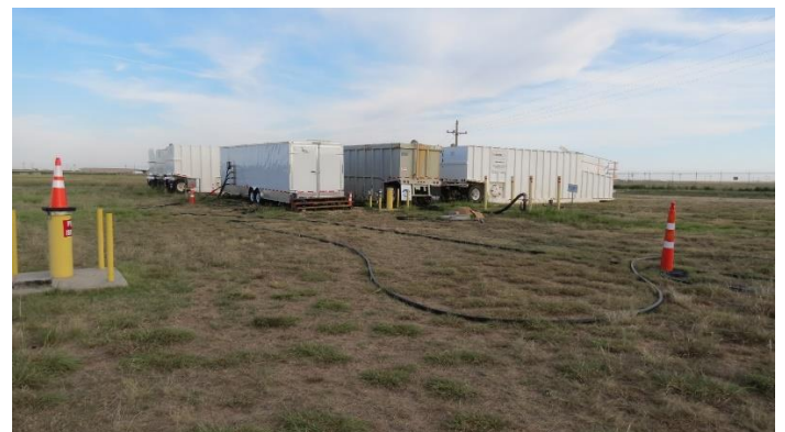
Injection Trailers at Zone 11 ISB
